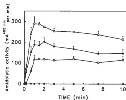
FIG. 1. Generation of amidolytic activity in mixtures of plasminogen with a 5-fold molar excess of staphylokinase (□, ■) or streptokinase (○, ●) in the absence (open symbols) or the presence (closed symbols) of  $\alpha_2$ -antiplasmin at a 5-fold molar excess over plasminogen. Amidolytic activity is measured with S-2251 (final concentration, 1 mM) after 50-fold dilution of samples. The data represent the mean  $\pm$  S.D. of three determinations.
